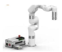
xArm 7 with 6 Axis Force Torque Sensor Fully Integrated Python API
